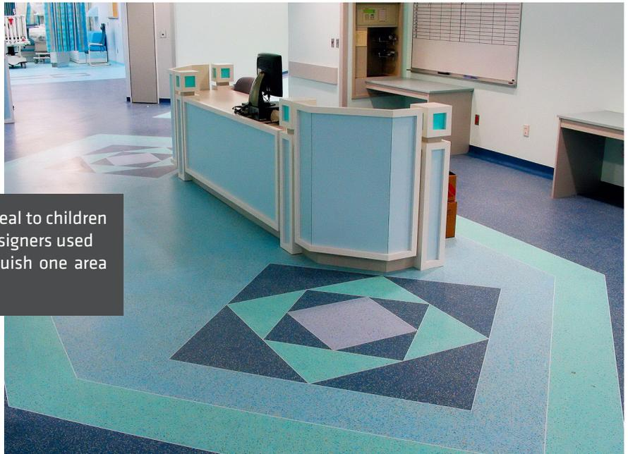
When she attended a "lunch and learn" sponsored by Stonhard, Mullins discovered Stonhard's Stonres RTZ, a stylized urethane floor system infused with multi-colored urethane aggregate chips to produce a durable and high-performance system while allowing intricate patterns and unique design capabilities. Stonres RTZ was the winning solution.
