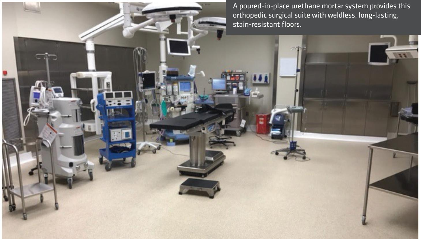
A poured-in-place urethane mortar system provides this orthopedic surgical suite with weldless, long-lasting, stain-resistant floors.
