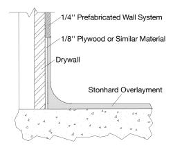
COVE BASE DETAIL with Pre-fabricated Wall System
