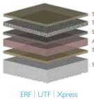
Stonhard Sealer (Two Coats) Stontec Flakes (Broadcast) Stontec Undercoat Aggregate (Broadcast) Stonhard Primer
