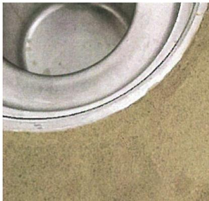
The installation of the round drain was waterproof after the test and no cracks were observed in the flooring material at the drain.
