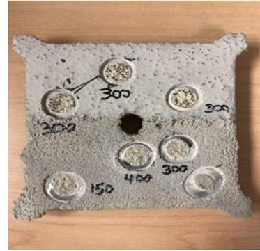
Figure 3: Stonclad UT on Natural and Sanicoat PolySto curbs
