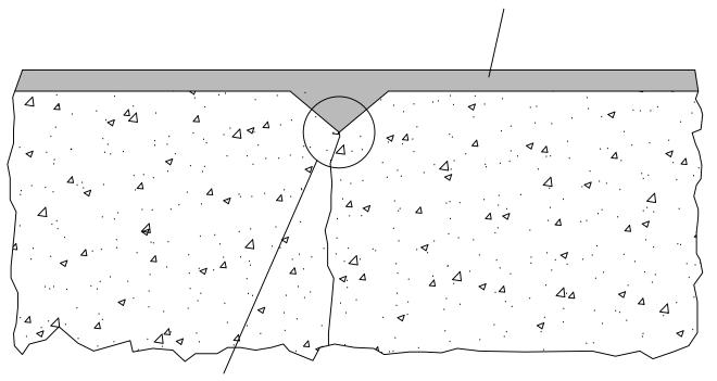
Joint routed out and pre-filled with mortar
